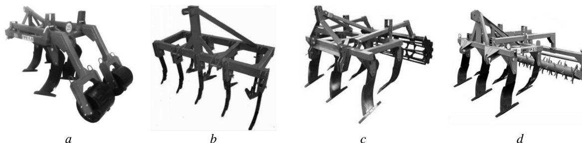
Fig. 1. Combined chisel-type deep cultivators: a – with smooth rollers; b – with cultivator tines; c – with a slatted roller-structure-forming; d – with a toothed roller-structure-forming
