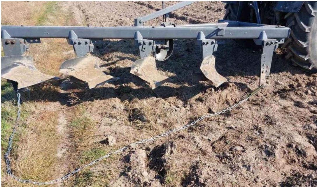
Fig. 14. Combined soil tillage unit consisting of: PLN-5-35 plow (modernized) and flexible chain subsoiler
