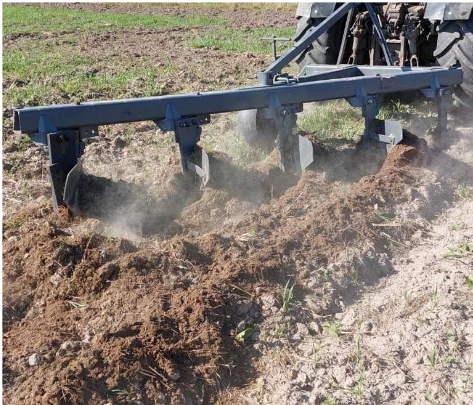
Fig. 17. Field testing of the combined soil tillage unit consisting of: PLN-5-35 plow (modernized) and flexible chain subsoiler
