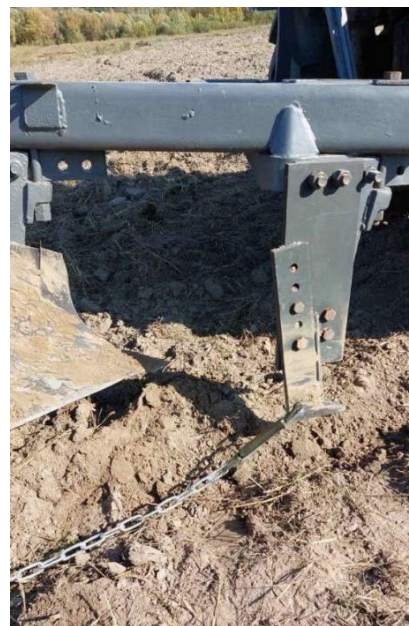
Fig. 14. Combined soil tillage unit consisting of: PLN-5-35 plow (modernized) and flexible chain subsoiler
